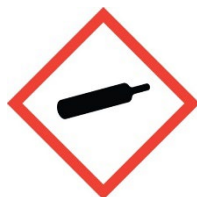
Gas Under Pressure
